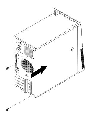
Figure 49. Reinstalling the computer cover
